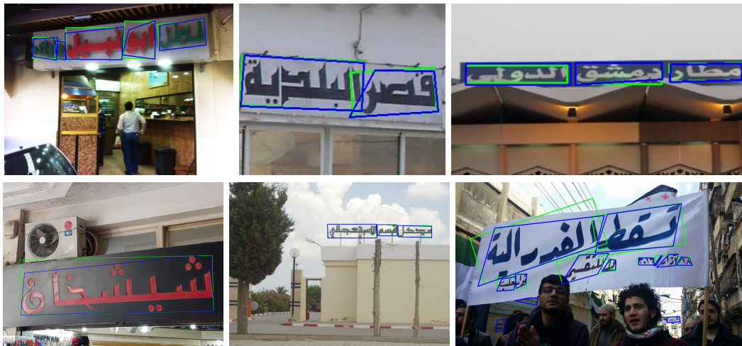
Fig. 5: Examples of bounding boxes predicted by a language-specific classification model (green) and their respective ground-truth annotation (blue).
